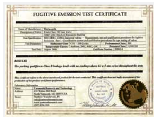
Emissions after 500 cycles at ambient and 350 °F Issued by Yarmouth Research and Technology Lab for 8 inch Class 300 Gate Valve After 500 cycles the measurement result was less than 50 ppm.
