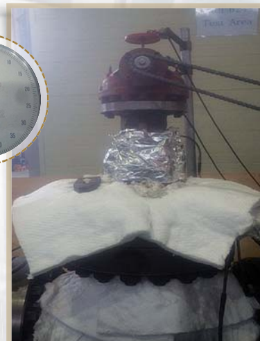
API 624 LFE TEST (A216-WCB, CL1500, 12" GATE, RF)
